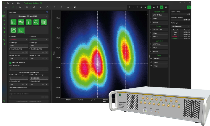
Fig. 1: Preliminary design of HydraHarp 500 L main unit together with PNR analysis and correction tools implemented in UniHarp software.
