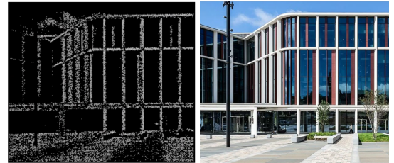
Fig. 2: The edges of shapes generated by the SPAD and RGC filter on the University of Glasgow's Advanced Research Centre (Left), compared to the ground truth image (Right).
